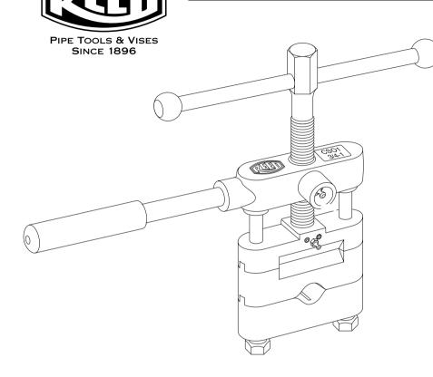
CSO1 <sup>3</sup>/<sub>4</sub>" - 1" (19-25 mm) CSO2 1 <sup>1</sup>/<sub>4</sub>" - 2" (32-51 mm) **Shutting off flow:** Assemble tool handle where desired. Unscrew the main feed screw. Lift and swing out dies to allow tube to seat between crimping dies. Swing dies back over the tie rods. Turn the feed screw to compress the tube using only enough pressure to shut off flow.
